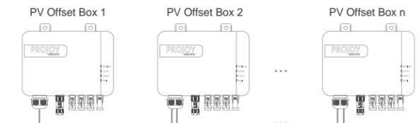
For multiple string inverters power stations, PROJOY PV Offset Box supports multiple sets in series, through one set of alternating power supply, and connects to up to 16 PROJOY PV Offset Boxes.
